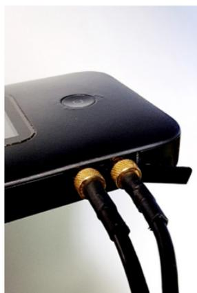
TS9 connections simply push in and pull out to remove. Please ensure when connecting or removing externally mounted antenna connectors ensure that this is done by holding the connectors themselves and not the cable to avoid any possible damage to the cabling.
